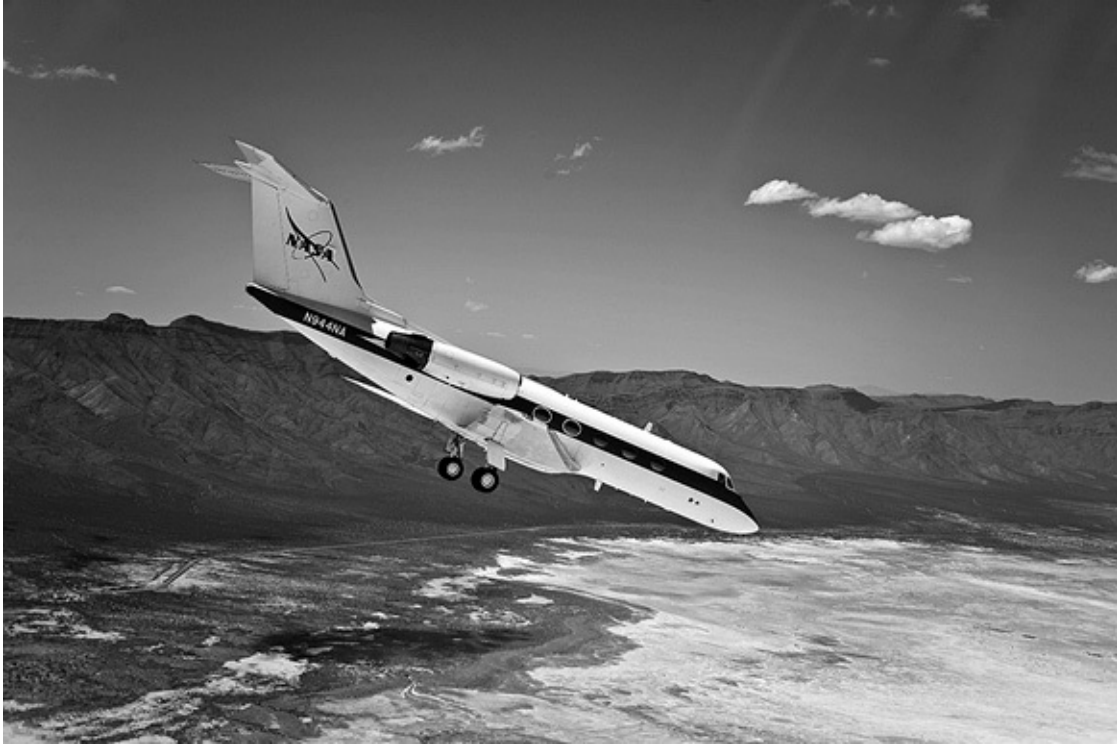
The unusual flight characteristics of the shuttle during approach and landing were simulated in the Shuttle Training Aircraft.
