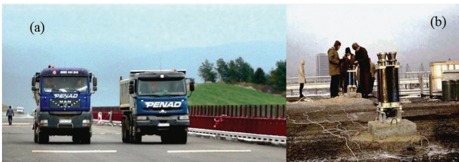
Figure 9. Testing load: (a) lorries traveling over the obstacles; (b) the PRE applied mainly on large bridge structure.
